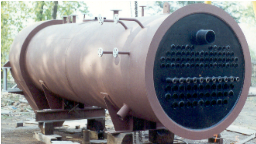
Shell for Waste Wood Fired, 2 Ton/Hr Boiler, Supplied to: - M/s. Shrinath Wood Industries, Yamunanagar
